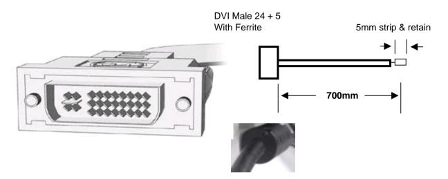
Cable: DVI cables feature mini-coax shielding, and tested to meet QXGA resolution (2048x1536).
