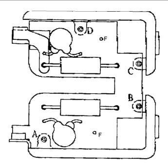
Solder only A, B, C, D: Resister + Capacitor connection. Point F : No solder
