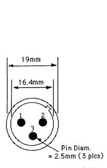
Pin 1, 3 connected to unmarked wire Pin 2 connected to marked wire
