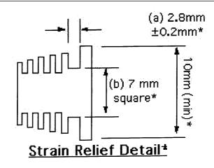
\* We do NOT want to create a new strain relief mold for this cable assembly The Strain relief should be a standard mold already used by the manufacturer (you) will adjust the hole in our product corresponding to dim (b) to match your standard strain relief. Contact Mobility and provide your drawings of your strain
