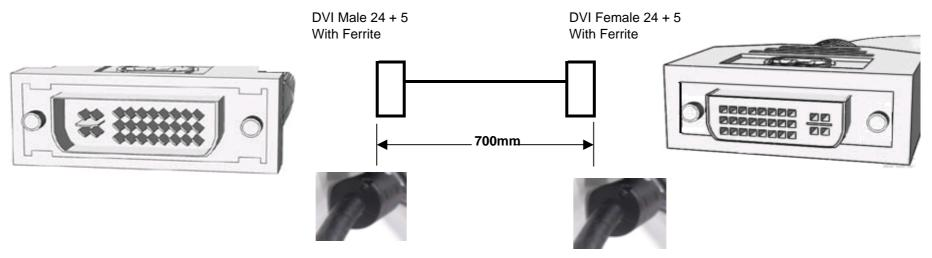
Cable : DVI cables feature mini-coax shielding, and tested to meet QXGA resolution (2048x1536).
